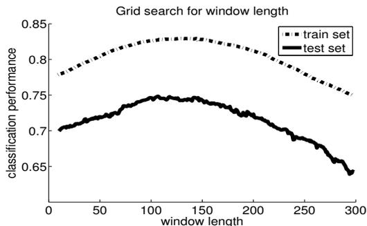
**Fig. 1.** Training (dashed) and test (solid) classification performance for various window lengths.
