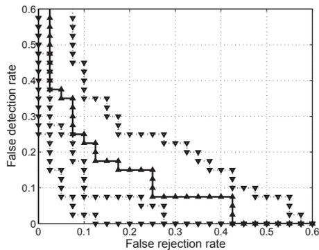
Fig. 2. DET curves for the class gunshot in tubestation noise, for the SNR values of 20, 10, 5, and 0 dB.
