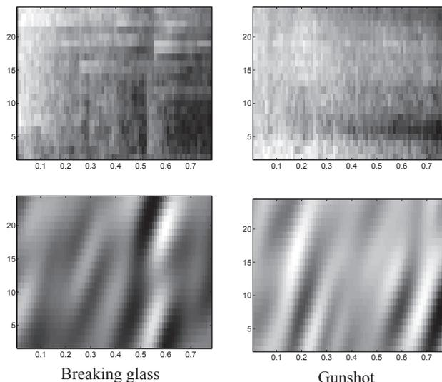
**Fig. 1.** log Mel-spectrogram (top) and output for one Gabor filter (bottom) for two recordings. The x-axis represents the time in s and the y-axis the Mel-frequency channels.
