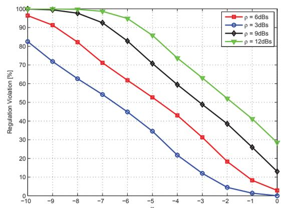
Figure 2. Regulation outage versus  $\alpha$  for different regulation constraints.
