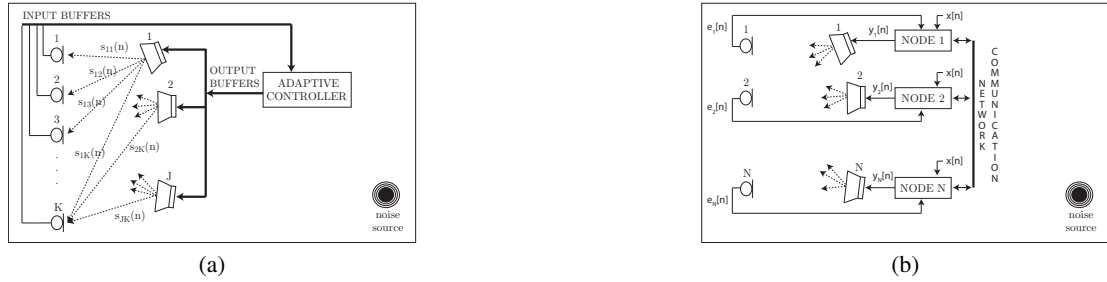
Fig. 1. Schemes of (a) a centralized ANC system, (b) a distributed ANC system with single-channel nodes.
