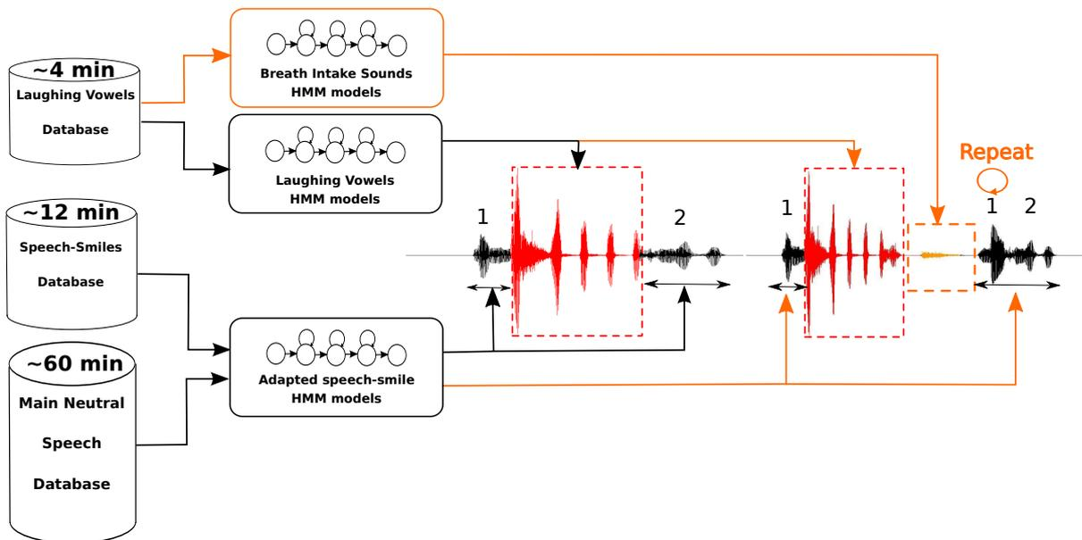
Fig. 1: HMM-based speech-laugh synthesis system pipeline and updates made on it for the purpose of this work (orange).
