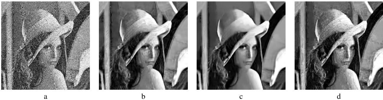
Fig. 5. Test image 19: a) noisy phase for  $\sigma_{\varphi_z}=0.2$ ,  $PSNR_{\phi}=26.9$  dB, b) phase reconstruction by CD-BM3D,  $PSNR_{\phi}=39.1$  dB, c) phase reconstruction by ImRe-BM3D,  $PSNR_{\phi}=39.8$  dB, d) phase reconstruction by BM3D,  $PSNR_{\phi}=37.8$  dB,.
