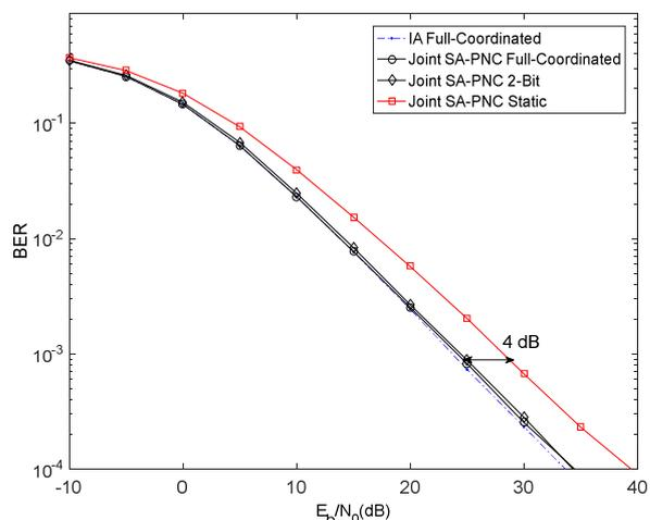
Fig. 3. BER Performance at the Small-cell System using QPSK modulation.
