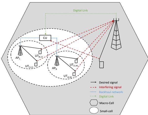
Fig. 1. System Model: Small-cells within coverage area of macro-cell.
