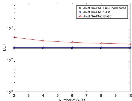
Fig. 4. BER Versus Number of small-cell UTs using QPSK modulation.
