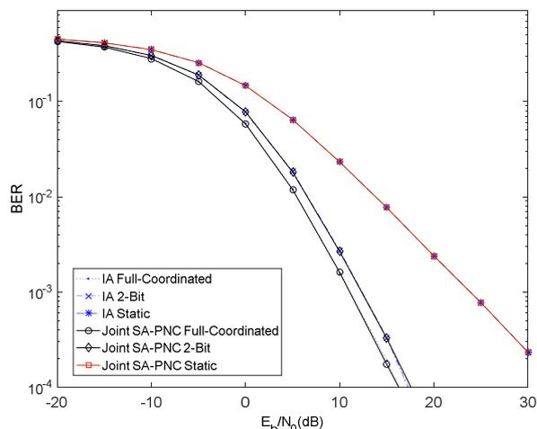
Fig. 2. BER Performance at the macro-cell System using QPSK modulation.
