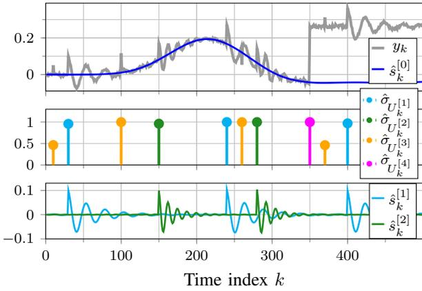
Fig. 2. Synthetic example of signal separation. For each signal component  $\hat{s}_k^{[\ell]}$ ,  $\ell \in \{0, \dots, 4\}$ , the average squared error is below  $10^{-5}$ .
