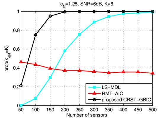
Fig. 3. Probabilities of correct detection versus the number of sensors.
