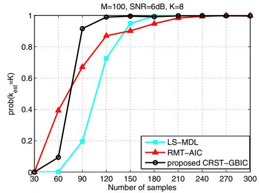
Fig. 2. Probabilities of correct detection versus the sample size.
