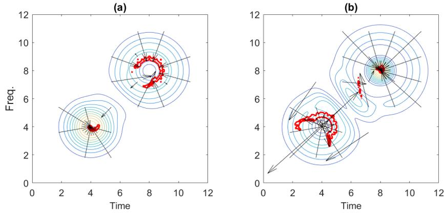
Fig. 1. Illustration of the spectrogram and the scaled reassignment of a signal with one Gaussian, (4, 4), and one second Hermite, (8, 8), signal component. The spectrogram is shown by the gradient lines. The arrows represent the reassignment of the signal energy and the red areas show the most energy dense areas in the ScRe-Spect; (a) Scaled reassignment with a Gaussian window; (b) Scaled reassignment with a second Hermite window.
