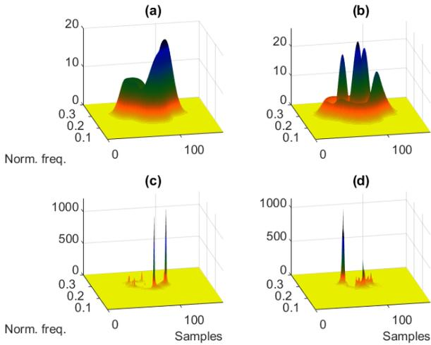
Fig. 2. Detection and time-frequency localisation of individual components in a multi-component transient signal; (a) The spectrogram with Gaussian window; (b) The spectrogram with second Hermite window; (c) The ScRe-Spect with Gaussian window; (d) The ScRe-Spect with second Hermite window.
