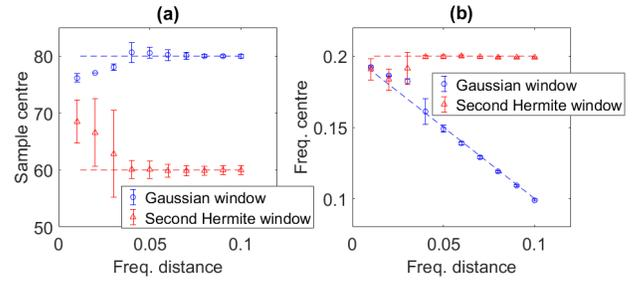
Fig. 4. The frequency distance between the two components in signal (19) is varied to get the average sample-frequency centres of the largest peaks in the ScRe-Spect with Gaussian and second Hermite window respectively, as well as a 95% confidence interval, obtained from 200 noise simulations. The true sample-frequency centres of both signal components are also marked; (a) The sample centres of the largest peaks; (b) The frequency centres of the largest peaks.
