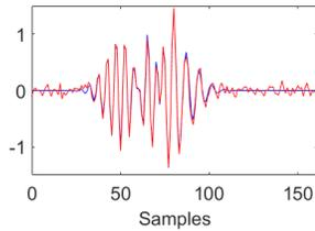
Fig. 3. Two component signal (19),  $f_1 = 0.14$ , with and without noise, SNR 15 dB.
