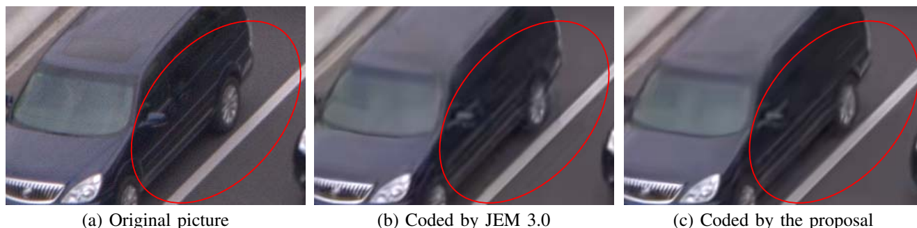
Figure 5. Subjective comparison between the original picture, the decoded pictures by JEM 3.0 and our proposed method. (The sequence ‘TrafficFlow’ is encoded at the QP value of 37 in all intra condition, and the cropped pictures in the resolution of 300x200 are illustrated for detail comparison)
