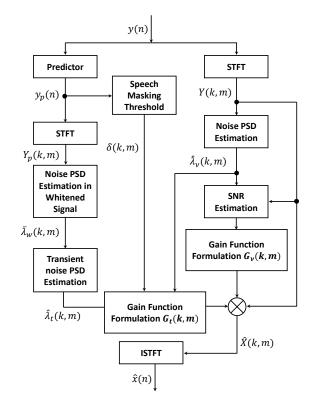
Fig. 1. Block diagram of transient and background noise suppression framework.
