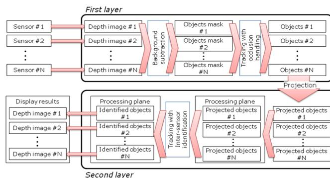
Fig. 1. Overall flow of the two-layer tracking method
