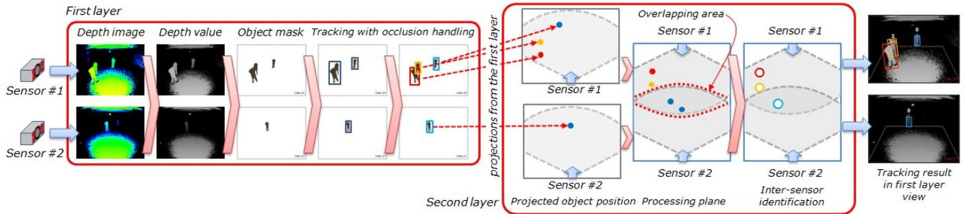
Fig. 2. Illustration of detection and tracking on the first layer and second layer involving two sensors.
