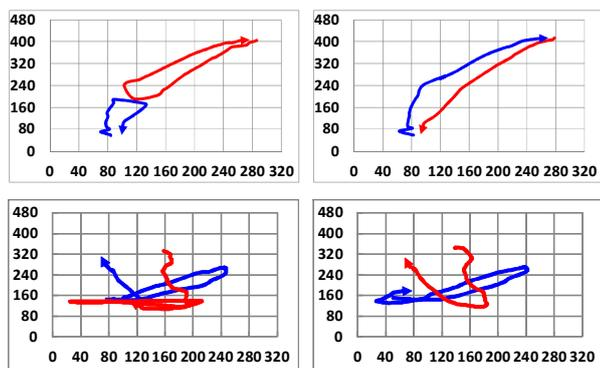
Fig. 5. Plots of trajectories of detected objects (left) without and (right) with occlusion tracking. Horizontal and vertical axes represent the width and the height of processing plane in pixels, respectively.
