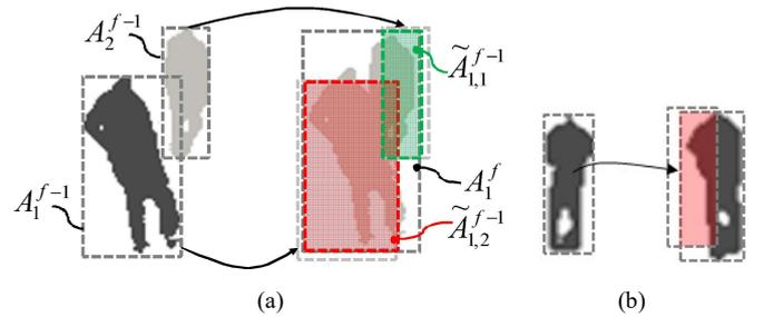
Fig. 3. (a) An example of occlusion detection between objects in current frame (right) and previous frame (left). (b) Example of intersecting area with only one object involved thus does not considered as occlusion.
