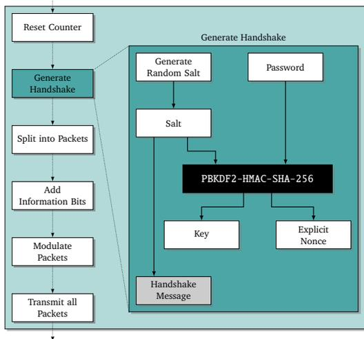
Fig. 1: Transmission of Handshake
