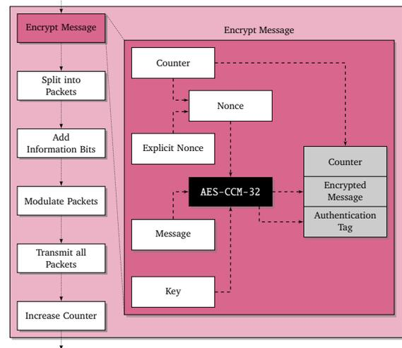
Fig. 2: Encrypted and Authenticated Transmission
