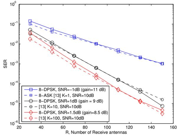
Fig. 5. SER comparison of DPSK constellation with energy based design.
