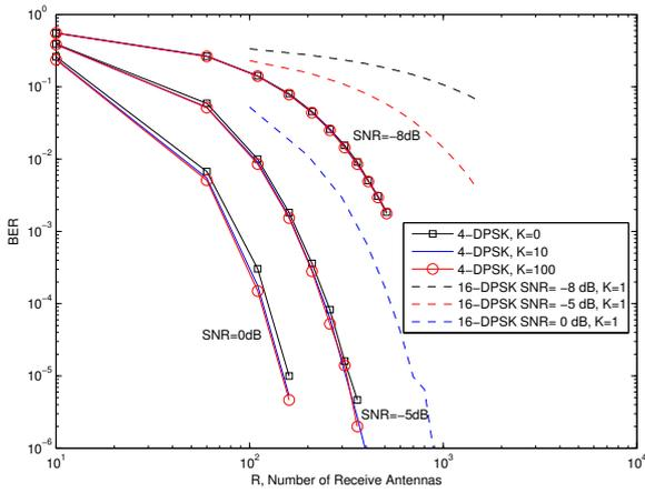
Fig. 3. Performance of 4-DPSK and 16-DPSK for several SNR and different  $K$  factors.
