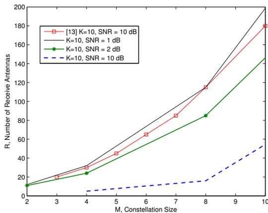
Fig. 7. Minimum number of receive antennas  $R$  for a target  $\text{SER} = 10^{-4}$  performance for two different constellation designs.
