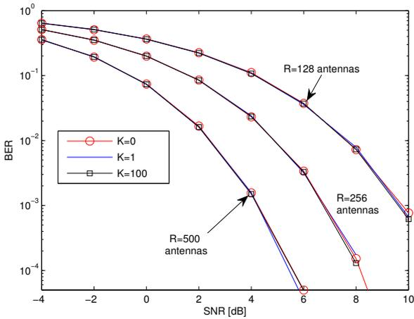
Fig. 4. Performance of 32-DPSK for different  $R$ .
