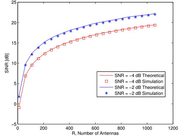
Fig. 2. SINR versus the required number of antennas.
