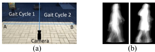
Fig. 6. Gait shadow sequences acquisition: acquisition location (a), example of appearance changes for the same user on different days (b).
