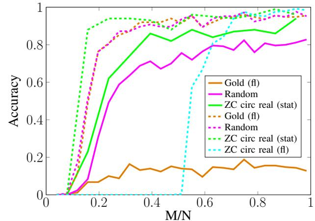
Fig. 5: Accuracy of the MWC with growing compression rate (K=6, 200 trials, OMP reconstruction algorithm), solid:10 dB ISNR, dashed: noiseless.
