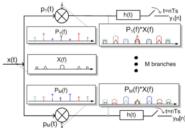
Fig. 1: Sensing process of the MWC.
