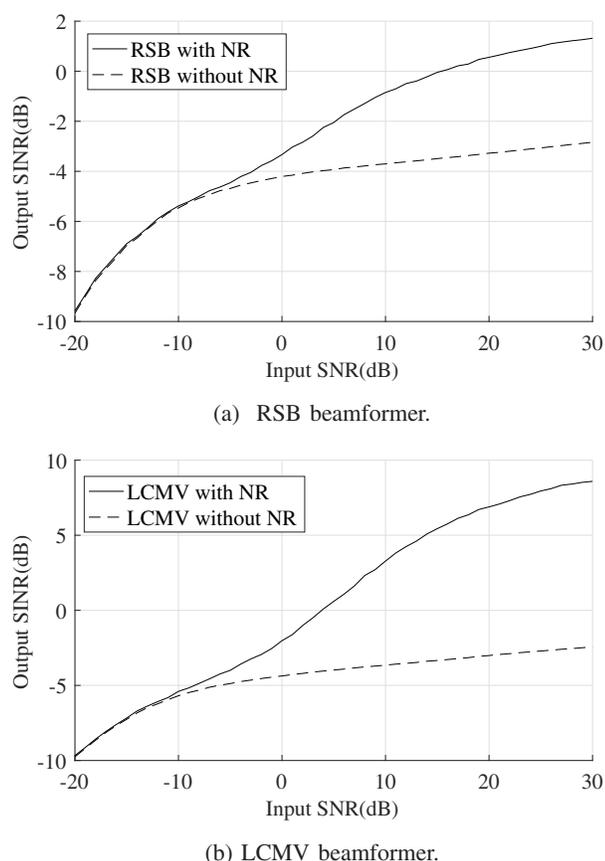
Fig. 4: SINR performance of both beamformers with and without the proposed noise reduction (NR) method for the sparse array specified in Table I.
