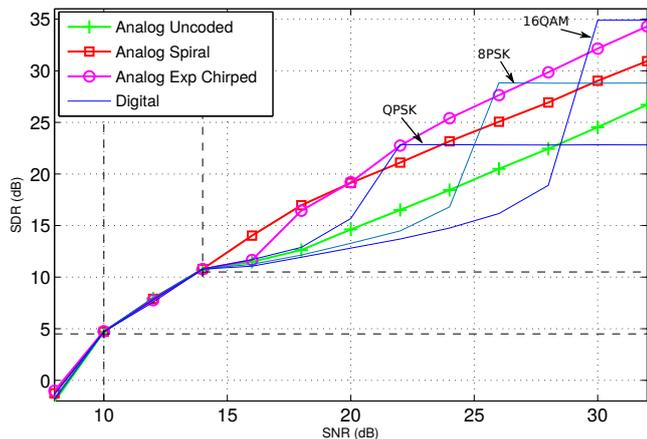
Fig. 5. Comparison of the the proposed HDA scheme to several digital approaches when considering three layers and an expansion factor  $R_l = 1$ .
