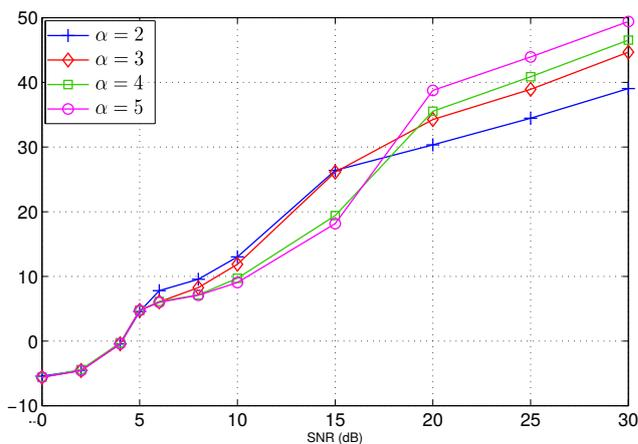
Fig. 4. Performance of analog chirped mappings for different values of  $\alpha$ .
