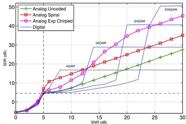
Fig. 3. Performance comparison between the HDA scheme with different mappings and the digital approaches with 2 layers and  $R_1 = R_2 = 1/2$ .
