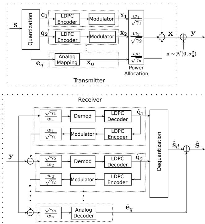
Fig. 2. Block-diagram of the proposed multilayer architecture.
