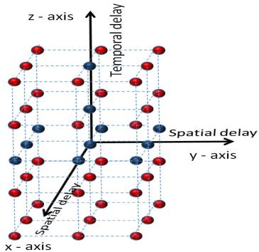
Fig. 2. Example of a DST for  $M_x = M_y = N = 3$ . Blue sensors shows the actual sensors, while the sensors shown in red depicts the virtual sensors.
