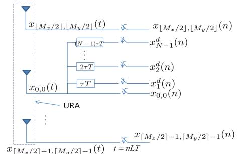
Fig. 1. Example of a multiple delay architecture considered in this paper. Notice that the delay channel network is added to the sensor placed at the origin.
