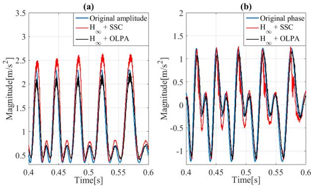
Fig. 2. Comparison between stochastic smoothness constraint and orthogonal Legendre polynomial for  $SNR = 0$  dB (a) Estimation of amplitude modulation (b) Estimation of the phase modulation
