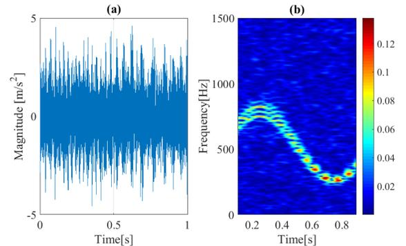
Fig. 1. Simulated signal with colored noise: a) Waveform b) Short-time Fourier spectrogram
