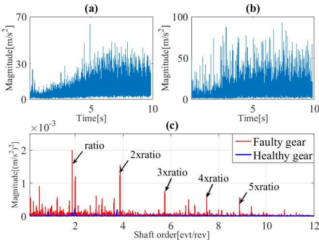
Fig. 5. Amplitude modulation: (a) Healthy case (b) Faulty case (c) Squared envelope order spectrum of amplitude modulation
