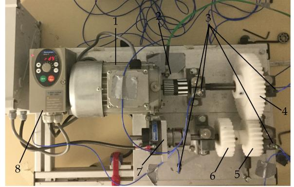
Fig. 3. Test rig: -1 Drive motor, -2 Optical encoder, -3 Accelerometer, -4 Healthy pinion, -5 Healthy gear, -6 Faulty gear, -7 Generator, -8 Speed variator
