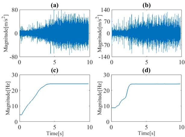
Fig. 4. Measurement signal: (a) Healthy signal (b) Faulty signal (c) Rotating frequency of healthy case (d) Rotating frequency of faulty case
