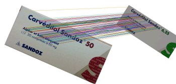
Fig. 14: RANSAC matching based on SIFT (#desc. = 1000, S1): different packages. Around 40% of matched descriptors. The difference is in the number of pills and active components.
