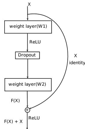
Fig. 2: Residual block used in this study.
