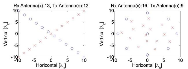
Fig. 3. Mills Cross array (left), curvilinear array (right)
