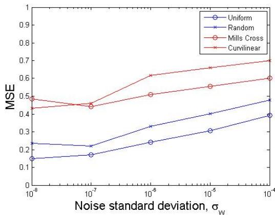
Fig. 5. MSE vs noise standard deviation for all topologies
