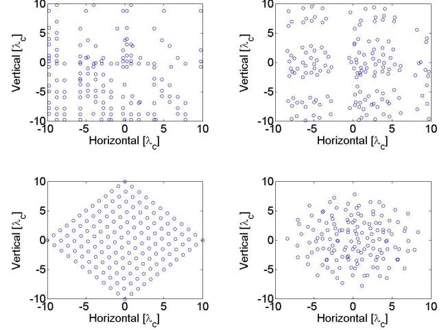
Fig. 6. Virtual arrays: for the design obtained with initially uniform array (upper left), for the design obtained with initially uniform array (upper right), for Mills cross array (bottom left), for curvilinear array (bottom right)
