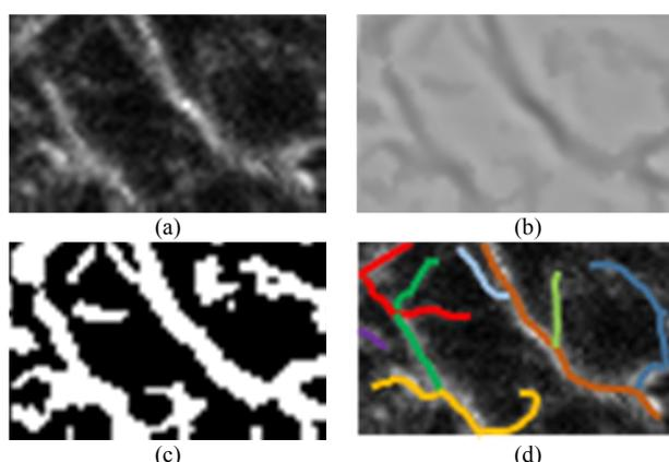
Fig. 5. Illustration of the main steps of the algorithm. (a) A middle z-slice crop from an image of a collagen hydrogel with 1 mg/mL concentration. (b) The response of the steerable filter. In this case, the fibers correspond to a negative response (i.e., dark values). (c) The binary mask corresponding to the sample collagen hydrogel network. (d) The reconstruction of individual fibers where each individual fiber has been labeled with a different color.
