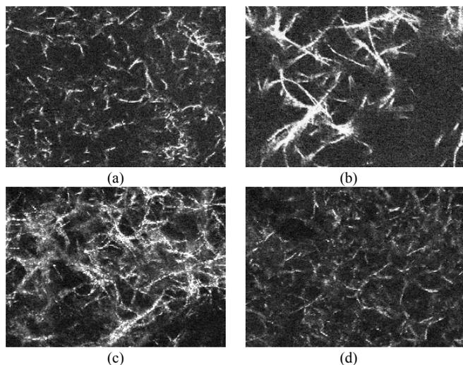
Fig. 3. Sample middle z-slice crops of size  $64.64\mu\text{m} \times 47.43\mu\text{m}$  from the confocal reflection microscopy images of the collagen hydrogel volumes polymerized on a microfluidic device. Concentration (mg/mL): (a) 1.0, (b) 1.5, (c) 2.0, and (d) 2.5.
