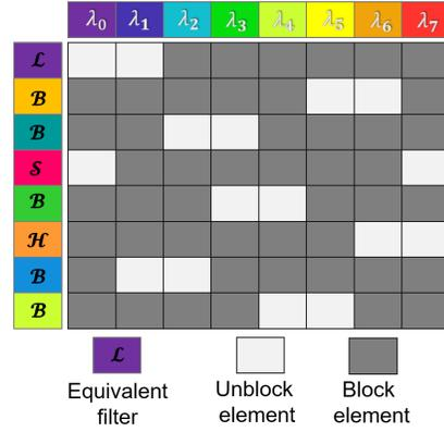
Figure 1: Illustration of the spectral responses of the set of optical filters. A maximal distance between unblock elements provides a minimal spectral correlation
