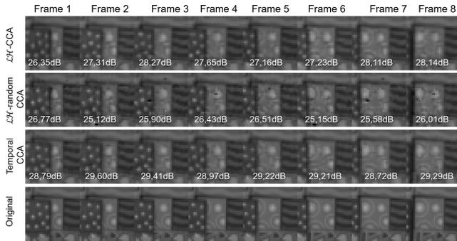
Figure 5: Preview reconstruction of the eight band by using the three coded apertures. Notice that the designed apertures achieves better quality reconstruction in terms of PSNR
