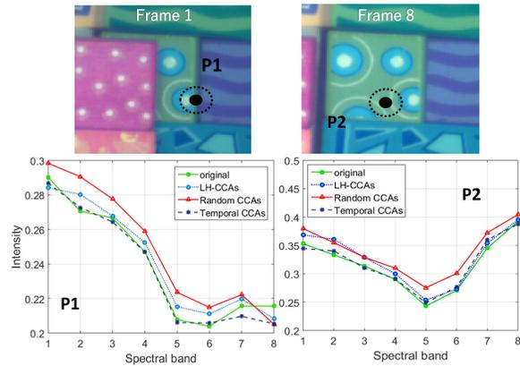
Figure 4: Spectral signature comparison for points P1 (frame 1) and P2 (frame 8) of the spectral video 1 using the  $\mathcal{L}\mathcal{H}$ -CCA, the  $\mathcal{L}\mathcal{H}$ -random CCA and the temporal CCA.
