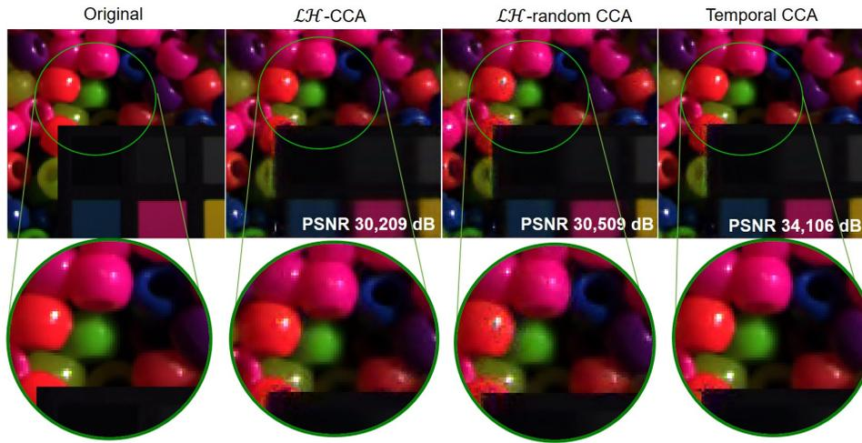
Figure 3: RGB representation of the original fifth frame of the spectral video 2 and the reconstructed frame using  $\mathcal{L}\mathcal{H}$ -CCA, the  $\mathcal{L}\mathcal{H}$ -random CCA and the temporal CCA.
