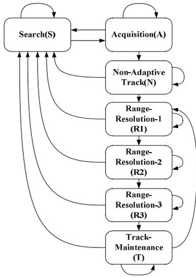
Fig. 2. Operating mode transitions of "Mercury" radar
