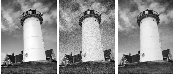
Figure 3: (Left) Original image ( 640 \times 480 pixels), (Middle) Image distorted with zero-mean Gaussian noise with variance 0.025 (PSNR -31 dB), (Right) Denoised image with \mu = 24.5 .
