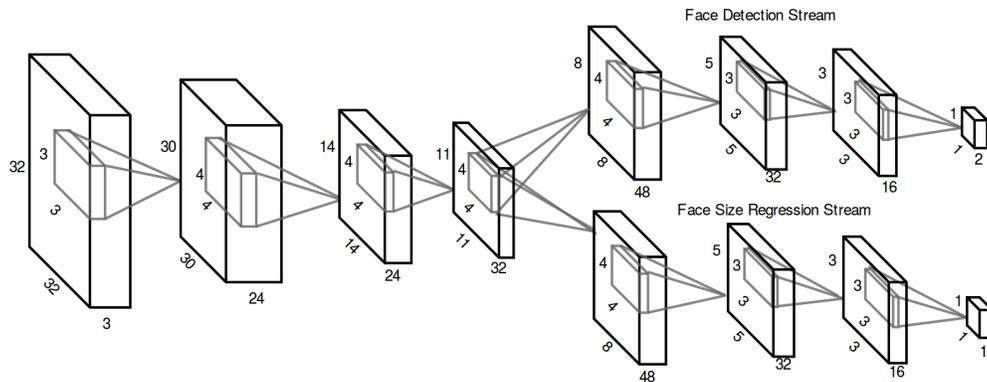
Figure 2. Architecture of the proposed two-stream convolutional face detector.
