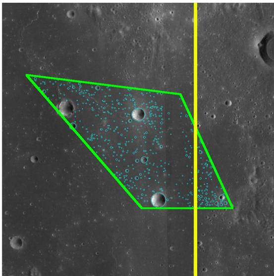
Fig. 5. Crater detections in area C3. The green polygon denotes the study area and the blue line separates the two different illumination directions.
