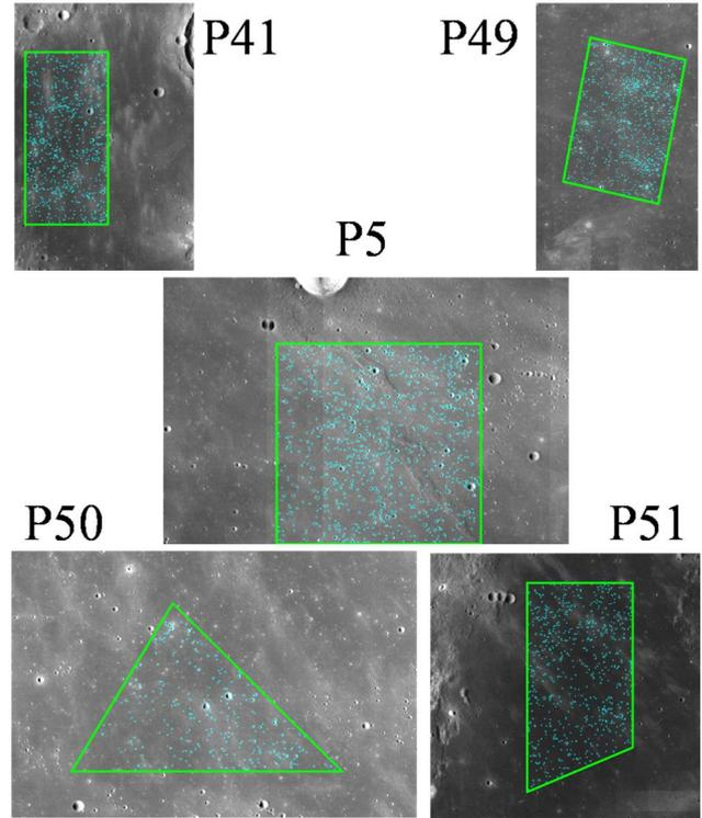
Fig. 4. Craters detected in the counting areas by the template matching based CDA in Oceanus Procellarum areas. The green polygons denote the counting areas.
