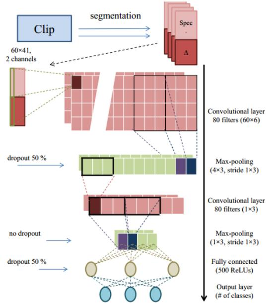
Fig. 3. CNN architecture for ESC used in this study. After [17].
