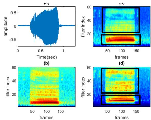
Fig. 2. Spectrographic analysis: (a) raw audio signal of cow sound, (b) Mel filterbank spectrogram, (c) Gammatone spectrogram, (d) TEO-Gammatone spectrogram. The regions indicated by black-boxes shows the differences between spectrum representation in (c) and (d).
