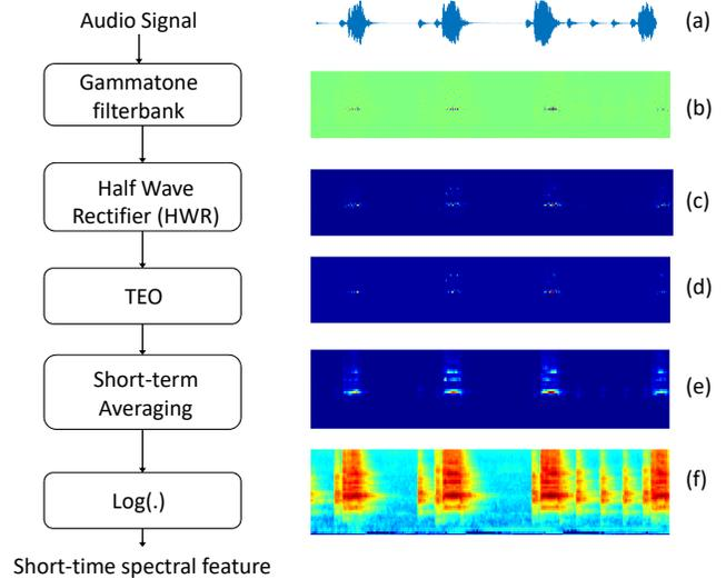
Fig. 1. Block diagram of the proposed features, (a) raw audio signal, (b) Gammatone filterbank response, (c) effect of the HWR on Gammatone filter responses, (d) TEO applied on each subband of Gammatone filterbank, (e) averaging of each subband filter response, (f) log-magnitude response of Gammatone TEO response.
