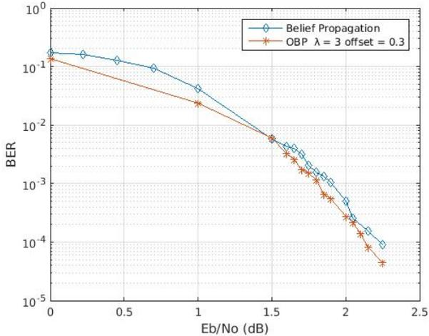
Fig. 1. Comparison of BP and BP  $\lambda$  min with offset
