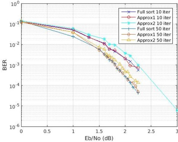
Fig. 8. Comparison of full sort with Approx1 and Approx2 for 10 iterations
