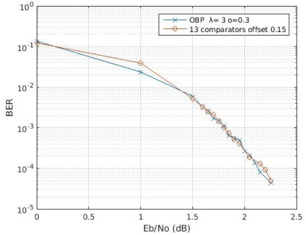
Fig. 6. Comparison of full sort with 13 comparator network (Approx1)
