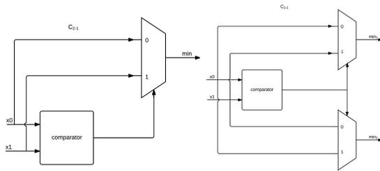
Fig. 9. Circuit for  $C_{2-1}$
