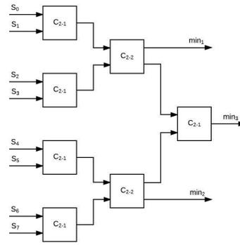
Fig. 12. Circuit that derives  $\lambda$ -minimum values with 7 comparisons
