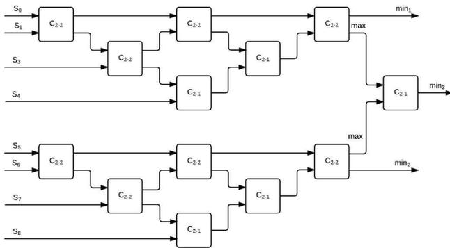
Fig. 11. Circuit that derives  $\lambda$ -minimum values with 13 comparisons
