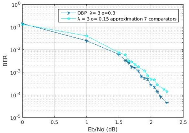
Fig. 7. Comparison of full sort with 7-comparator network (Approx2)
