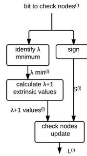
Fig. 2. Architecture of Check node process
