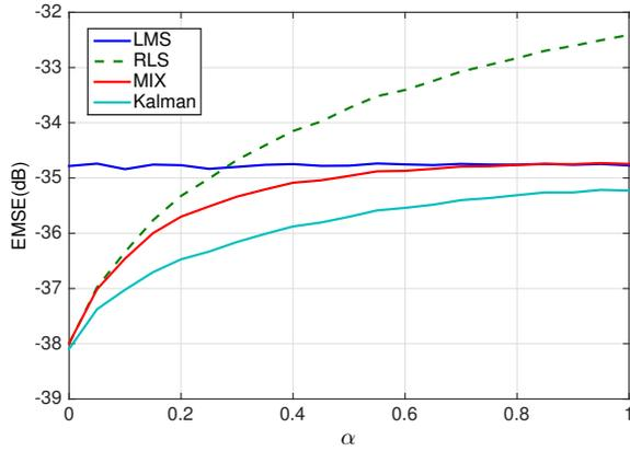
Figure 2. Simulated steady-state EMSE for LMS, RLS, their convex combination and KF, when  $\mathbf{Q}_n$  smoothly changes between  $\mathbf{R}_u$  and  $\mathbf{R}_u^{-1}$ .
