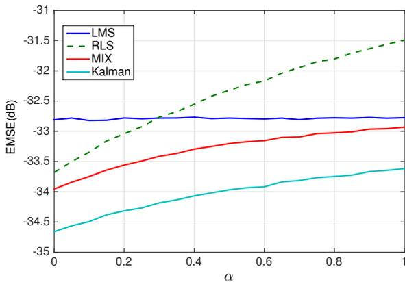
Figure 3. Simulated steady-state EMSE for LMS, RLS, their convex combination and KF, when a random perturbation is added to  $\mathbf{Q}_n$ .
