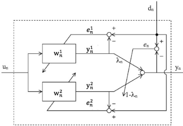
Figure 1. Block diagram of an adaptive convex combination of two transversal filters.
