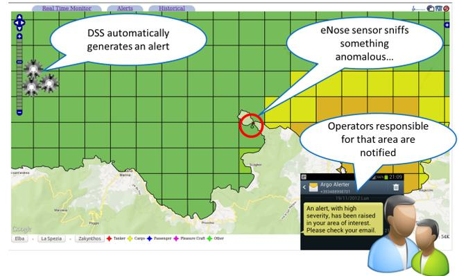
**Fig. 2.** The interface during field tests showing an event from an eNose sniffing; transmitted to the MIS, the DSS generates a preliminary alert, and operators notified
