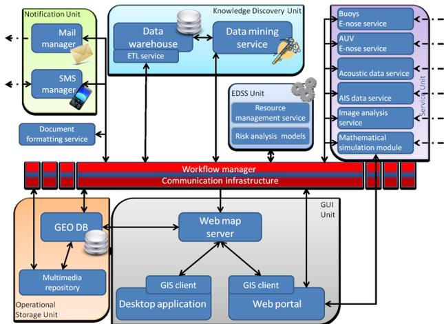
**Fig. 1.** The detailed architectural design of the MIS for environmental monitoring.
