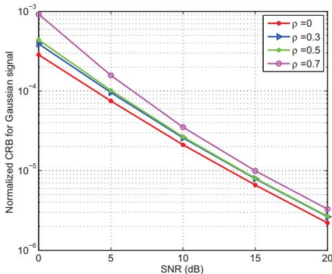
Figure 2. Gaussian CRB versus SNR with different orthogonality levels.
