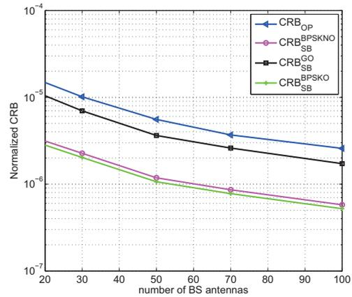
Figure 4. Normalized CRB versus number of BS antennas  $N_r$ .
