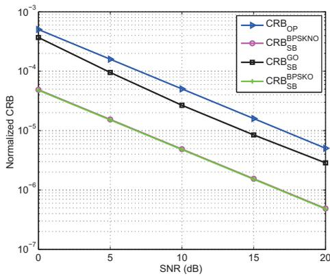
Figure 1. Normalized CRB versus SNR.
