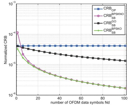
Figure 3. Normalized CRB versus number of OFDM data symbols  $N_d$ .
