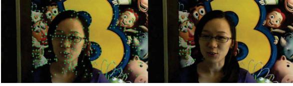
Fig. 2. Example on the close_person video (frame 100). On the left frame are all trajectories detected by the KLT tracker, and on the right are the selected trajectories. All trajectories corresponding to the moving woman have been removed.
