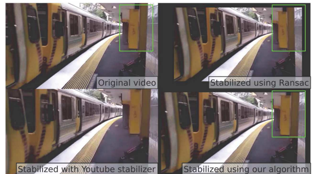
Fig. 4. Example on the 14_object video (frame 68). On the upper left is the original video, on the upper right the result of the RANSAC algorithm, on the lower left the results of the Youtube stabilizer and on the lower right the result of our algorithm. Cropped areas are displayed in black for RANSAC and our method. Youtube stabilizer automatically resizes the video.
