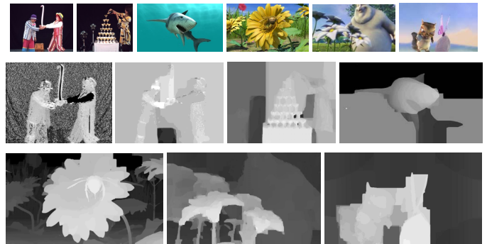
Fig. 4. 1D multi-view images (from top left: Pantomime, Champagne Tower, Shark, Bee, Flowers, Butterfly), depth maps estimated by matching error only (middle left) and with Graph-Cuts smoothing (others) [7][8]
