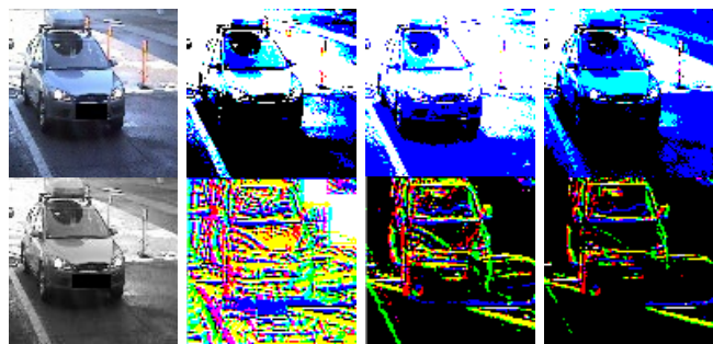
Figure 1. Input binarization with RGB Thresholding (first row) and LBP (second row).
