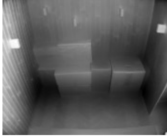
Fig. 1 Distance map with stretched value range representing a packaging scene. Lighter pixel values represent points closer to the scanner.
