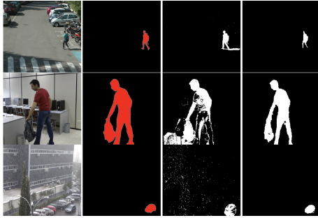
Fig. 2. Examples for the evaluation of the mask through the mask refinement method. First column: Input images. Second column: Corresponding annotation. Third column: Input mask obtained by MOG2. Forth column: Mask generated by the mask refinement network.
