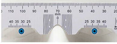
Fig. 6: The calibrated ruler used as the ground-truth for the pupil diameter measurement.
