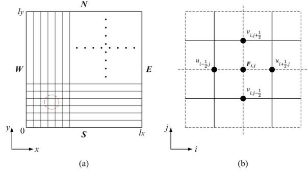
Fig. 1. (a) Illustration of the 3D flow in the  $xy$  plane and boundary symbols. This flow domain corresponds to one slice of the image volume under registration. (b) Illustration of staggered grids for the triple  $\mathbf{F}$ ,  $\mathbf{u}$  and  $\mathbf{v}$  in a grid cell with respect to the arbitrarily circled voxel in (a).
