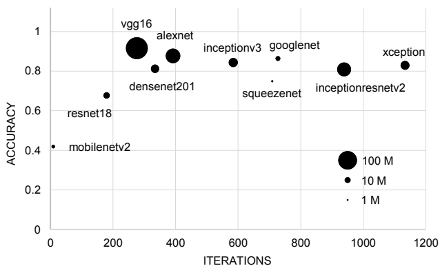
Fig. 4. Mean accuracy versus iterations of top performers architectures across ten folds for batch size: 8. 1M = 1 million. Iterations to reach best accuracy averaged across ten folds of the baseline design (train set = 90%)
