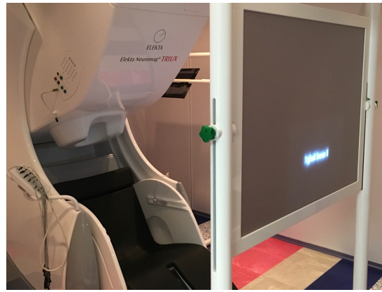
Fig. 1. The MEG machine housed inside a magnetically shielded room (MSR)
