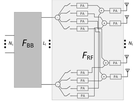
Fig. 1. Simplified architecture for Hybrid MIMO beamforming with analog switches, combiners, and splitters.
