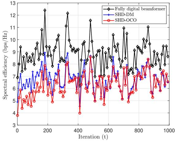
Fig. 3. Spectral efficiency achieved by fully digital beamformer, SHD-DM, and SHD-OCO for a 25 MIMO system.
