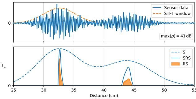
Fig. 6. An example of processing data from the Acconeer A1 sensor. The top plot shows the data and the manually matched window. The bottom plot shows the slice of the spectrogram (S), binned RS, and SRS, matching the frequency of the signal. The spectrogram has been scaled up for a better view.
