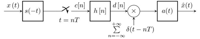
Fig. 1. Sampling and reconstruction of a signal in a shift-invariant space.
