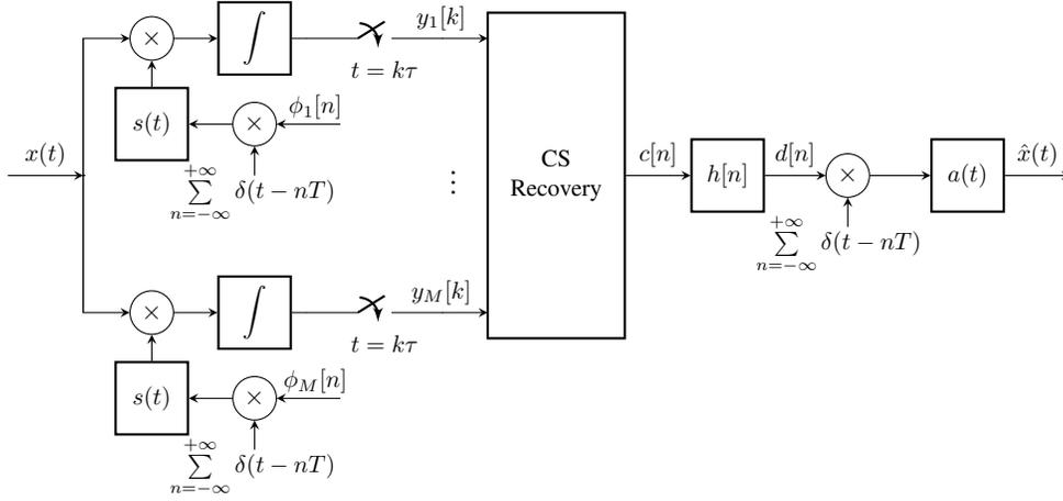
Fig. 3. Compressive sensing of an analog signal in a shift-invariant space with  $B_0$ -spline sampling kernel  $s(t)$  and a discrete-time correction filter  $h[n]$ .
