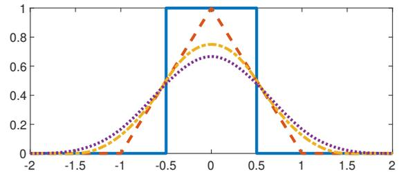
Fig. 2. The centered  $B_p$ -spline basis functions of degrees  $p = 0$  to 3. As  $p$  increases, the basis functions flatten out and their support expands.
