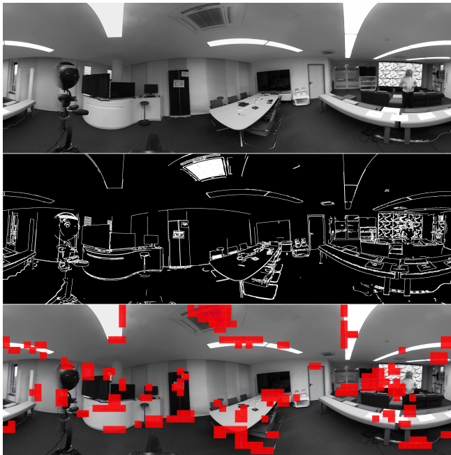
Fig. 1. Illustration of the algorithm workflow. Top: input image, middle: binary edge image, bottom: blocks from which the blurriness is calculated. Best viewed in color.
