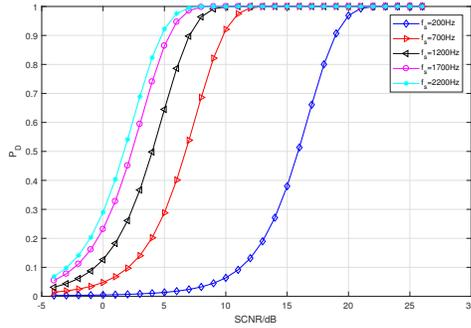
Fig. 2:  $P_D$  for GQEA method for different  $f_s$  for a cloud MIMO radar with  $M = 2$  transmitters and  $N = 3$  receivers.
