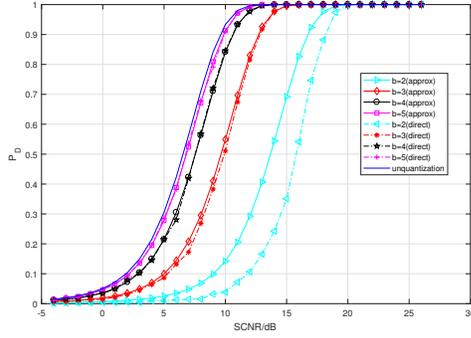
Fig. 1:  $P_D$  for direct analysis and GQEA method for different  $b$  for a cloud MIMO radar when sampling rate  $f_s = 600\text{Hz}$ .
