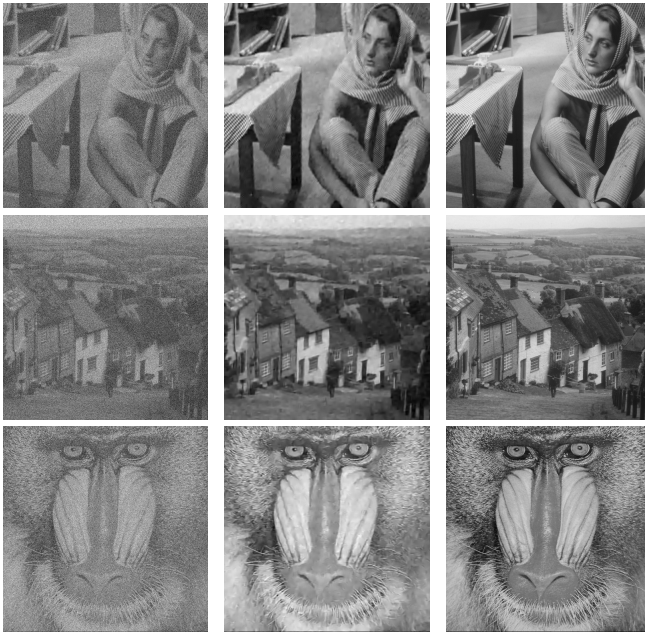
Figure 2. Denoising ( \sigma = 40 ) results obtained by using BBG-SVA. From left to right are the noisy, the denoised and the original images.
